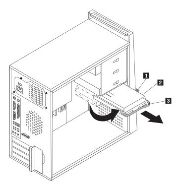
Figure 18. Removing the primary hard disk drive
